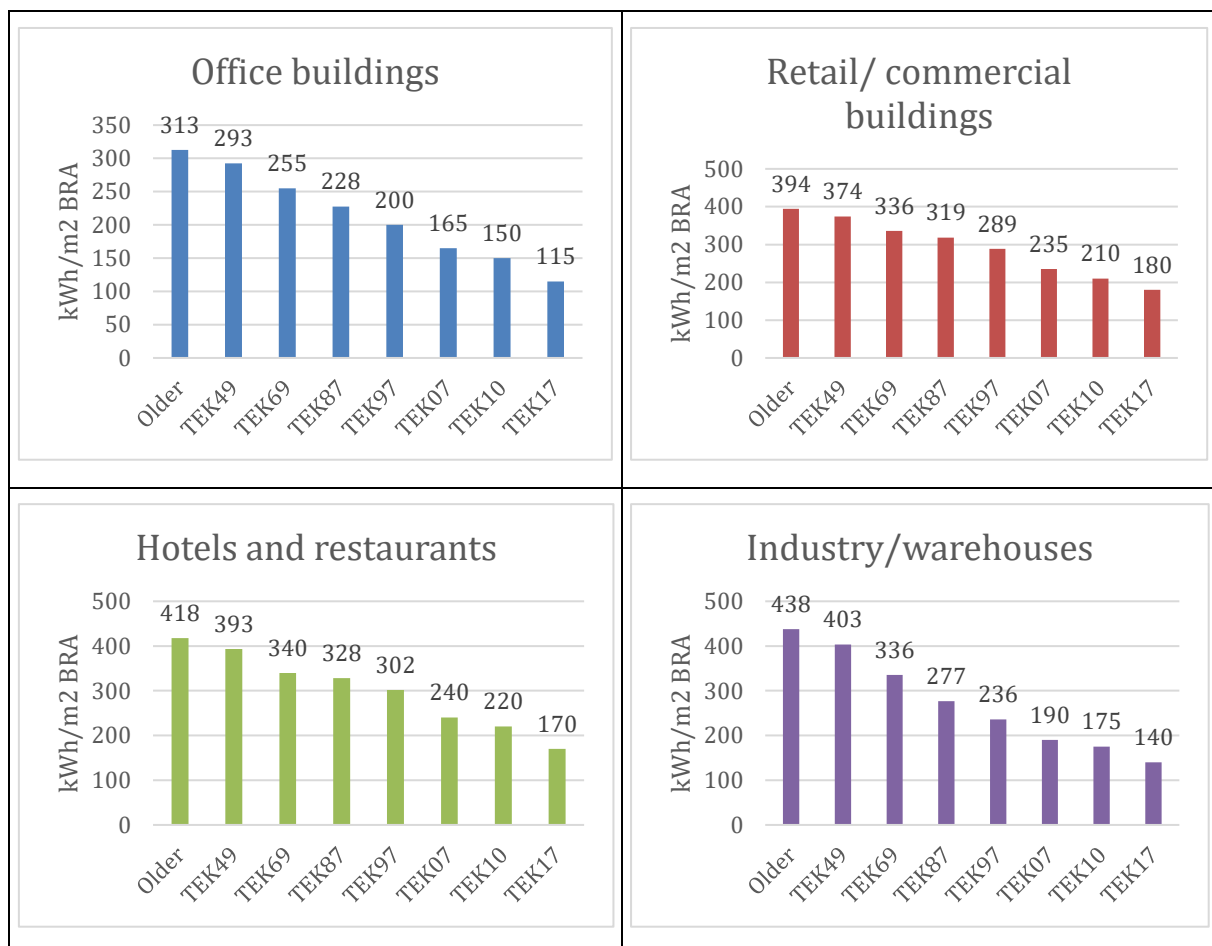
Figure 17 Development in calculated specific net energy demand based on building code and building tradition (Multiconsult, simulated in SIMIEN)
